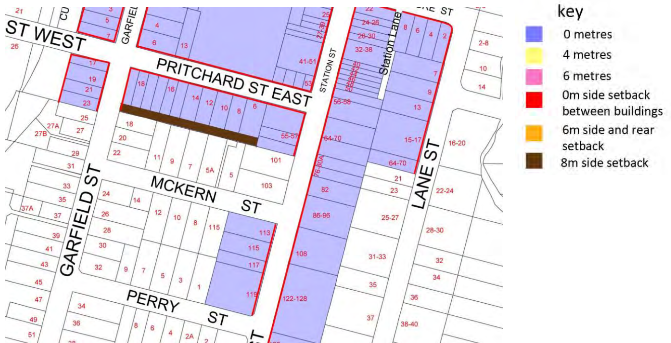
Figure 11- extract from Holroyd DCP 2013 indicated 8m setback for Pritchard Street East properties
